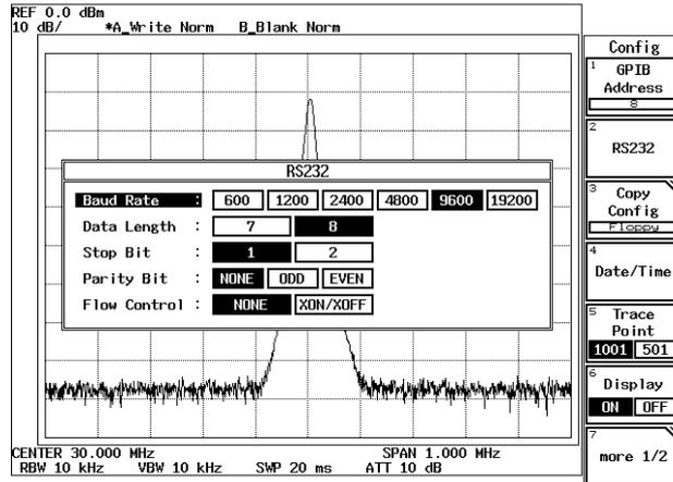
Figure 5-5 Parameter Setup
