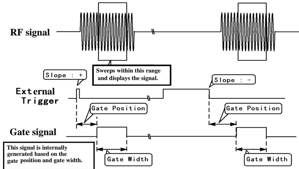
Figure 4-7 Generating the Internal Gate Signal
