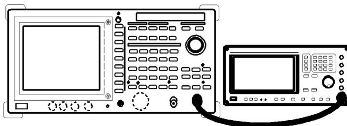
**Figure 2-53 Measuring Burst Signal in Separate Screen Mode**
