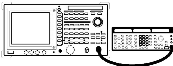
**Figure 2-49 Measuring AM Signal in Separate Screen Mode**
