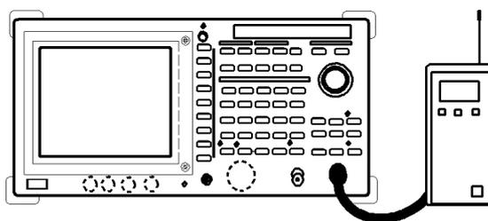
**Figure 2-102 Setup Measuring Adjacent Channel Leakage Power**
