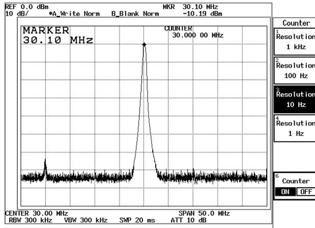
Figure 2-28 Frequency Counter Measurement (Resolution: 10 Hz)
