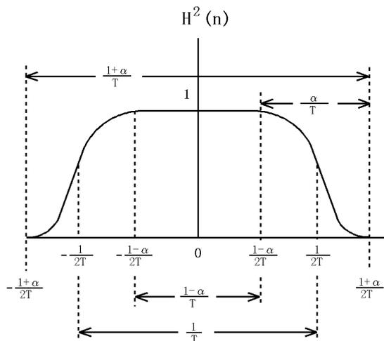
**Figure 4-5** Characteristics of the Root Nyquist Filter
