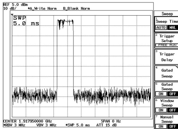
Figure 2-113 Burst Signal in the Time Domain
