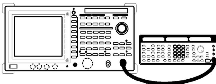
**Figure 2-121 Setup for Measuring the Harmonic Distortion**
