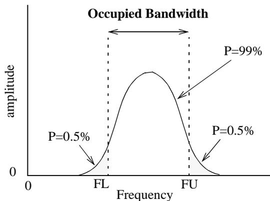
**Figure A-5 Occupied Bandwidth****Quasi Peak Value Measurements**
