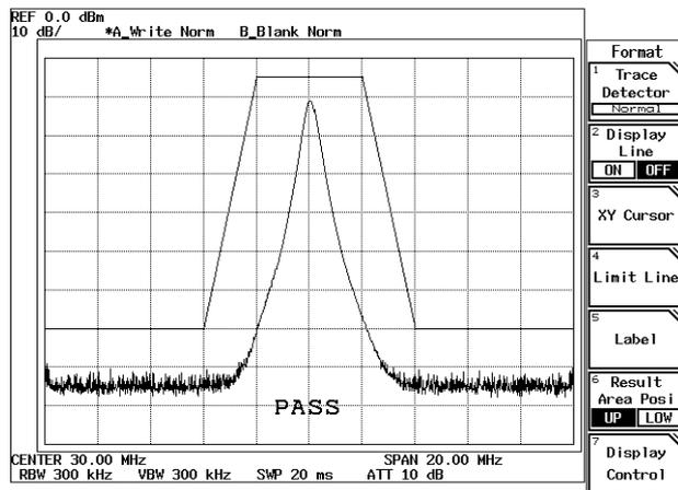
Figure 2-77 PASS/FAIL Result using Limit Line 1
