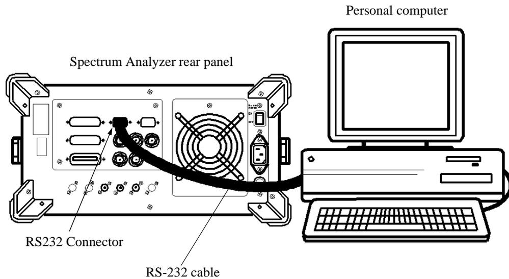
**Figure 5-6 Connection Between the Controller and the analyzer**
