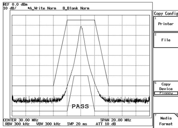
Figure 2-78 PASS/FAIL Result using Limit Lines 1 and 2
