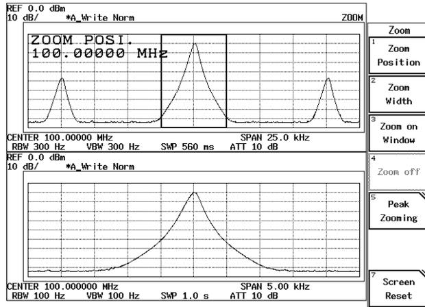
Figure 2-51 Displaying the Trace in Separate Screen Mode
