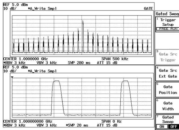
Figure 2-107 Burst Signal Displayed in Split Screen Mode
