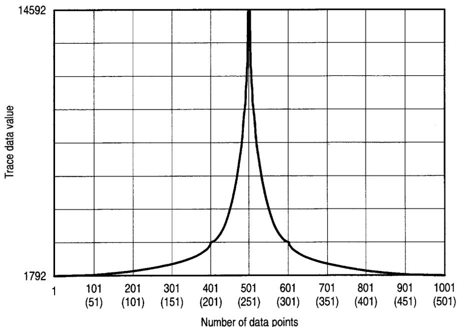
**Figure 5-4 Relationship between Screen Graticule and Trace Data**
