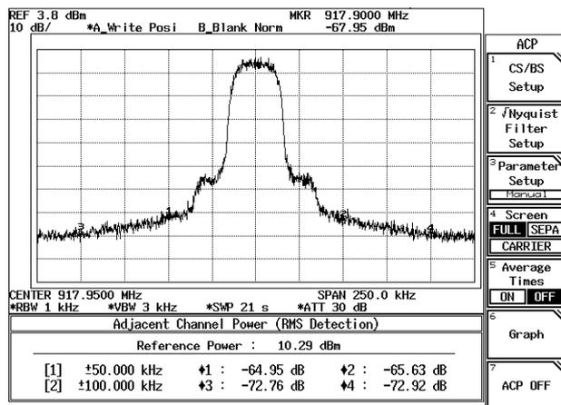
Figure 2-99 ACP Measurement Display in Full Screen Mode
