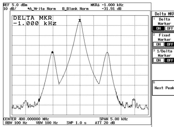
Figure 2-133 AM Signal with Low Modulation Factor
