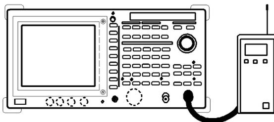
**Figure 2-85 Setup for Measuring the Total Power**
