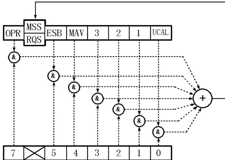
Figure 5-3 Structure of the Status Byte Register
