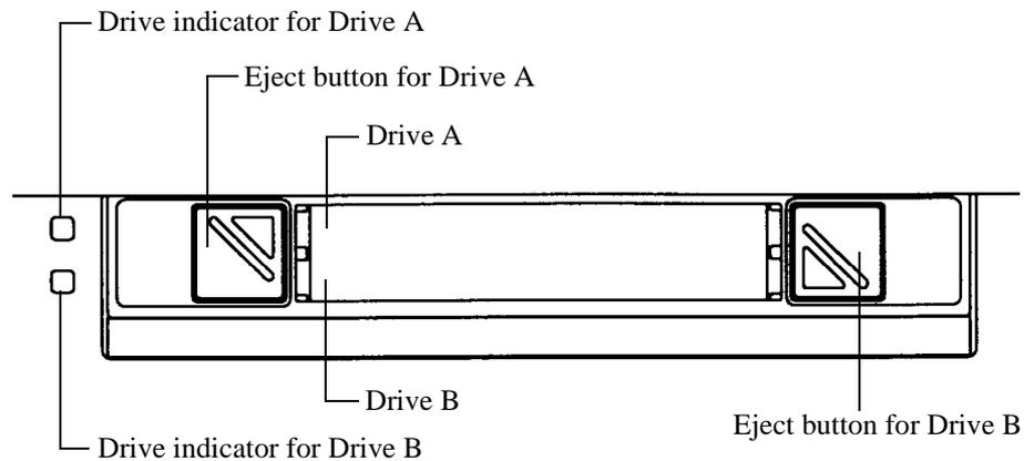
**Figure 2-158 Slots in the Memory Card Drive**
