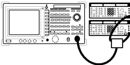
**Figure 2-37 Setup for Measuring Two Signals Separately**
