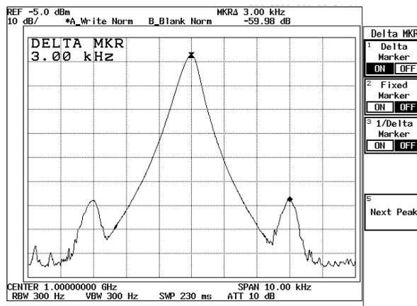
**Figure 2-138 Modulation Frequency of the FM Signal**
