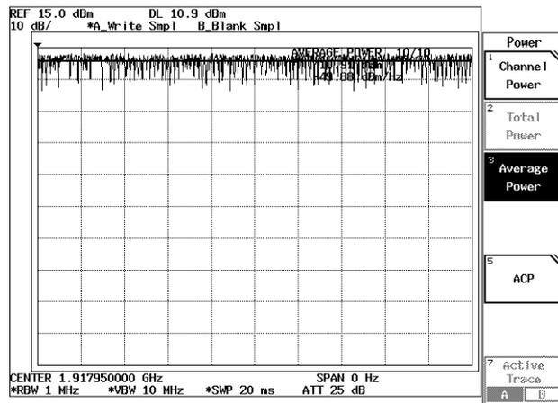
Figure 2-83 Result of an Average Power Measurement
