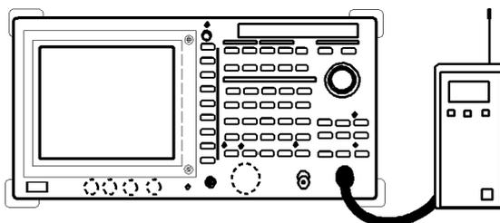
**Figure 2-80 Setup for the Average Power Measurement**
