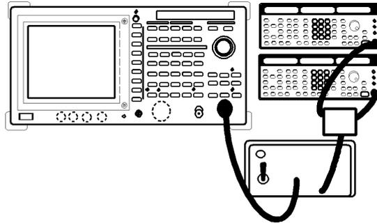
**Figure 2-128 Setup for Measuring the Third Order Intermodulation Distortion**
