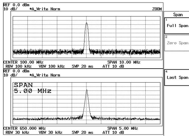
Figure 2-66 Setting for the Lower Screen in Separate Screen Mode
