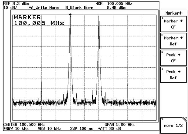
Figure 2-130 Third Order Intermodulation Distortion (Peak → Ref)
