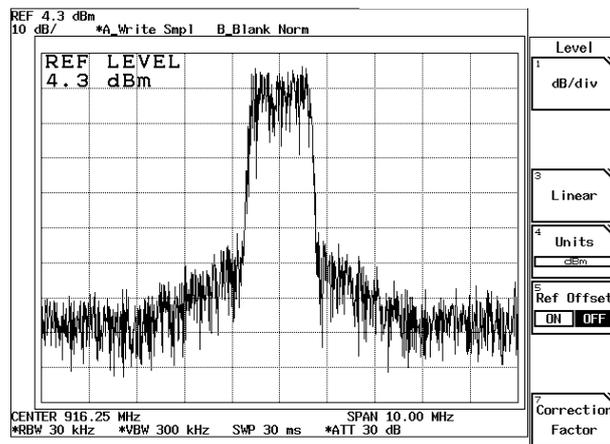
Figure 2-86 Setting Conditions for the Total Power Measurement
