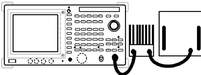
**Figure 2-141 Setup for Measuring Pulsed RF Signal**
