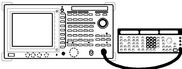
**Figure 2-46 Measuring AM Signal in Separate Screen Mode**
