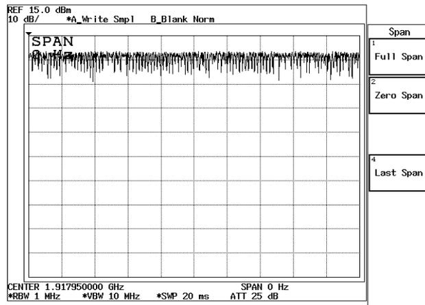
Figure 2-82 Setting Measurement Conditions for Average Power Measurement
