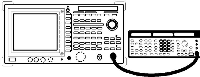
**Figure 2-41 Setup for Verifying the Dynamic Range**
