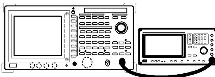
**Figure 2-106 Setup for Measuring a Burst Signal**
