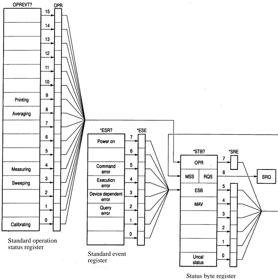
Figure 5-2 Details of the Three Status Registers
