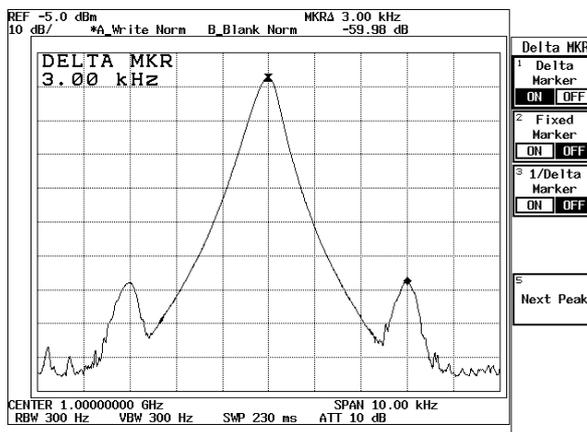
Figure 2-140 FM Signal with Low Modulation Index
