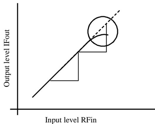
Figure 4-2 Relationship between the Input and Output of the Mixer
