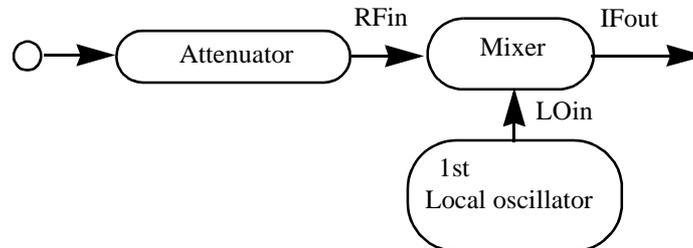
Figure 4-1 Input Section Block Diagram
