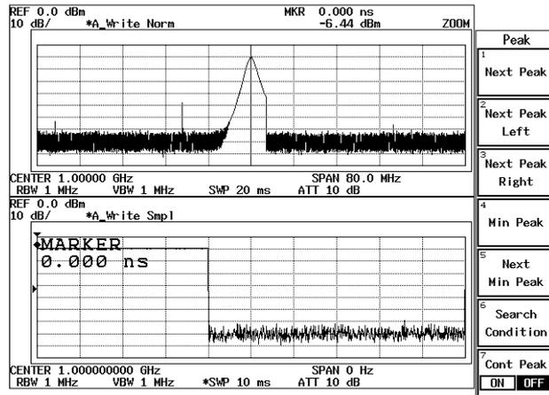
Figure 2-61 F/T Function Displayed in Separate Screen Mode
