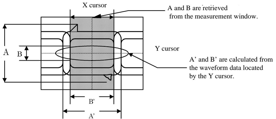
**Figure 4-9 Eye Opening Calculation (Using the Measurement Window)**
