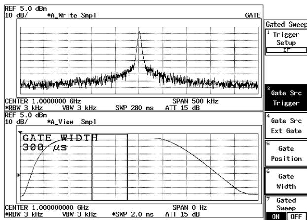
Figure 2-109 Burst Signal by Use of the Gated Sweep (Separate Screen Mode)
