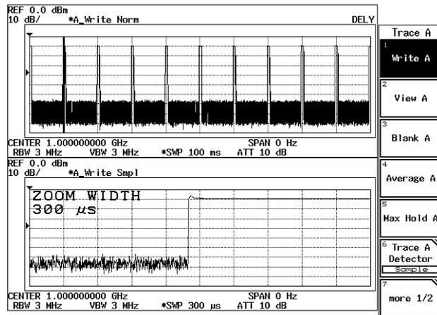
Figure 2-57 Observing the Leading Edge in the Separate Screen Mode
