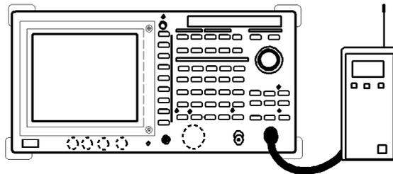
**Figure 2-88 Setup for Measuring the Total Power**
