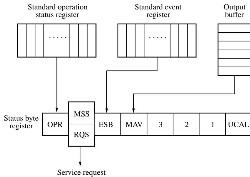
**Figure 5-1 Arrangement of the Three Status Registers**
