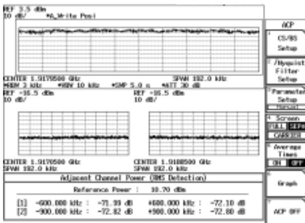
Figure 2-105 Measurement Result in ACP Separate Screen Mode
