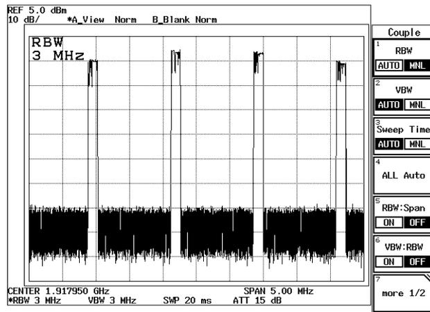
Figure 2-112 Burst signal in the frequency domain
