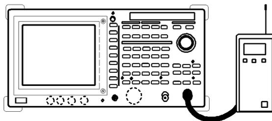
**Figure 2-93 Setup for Measuring the Occupied Bandwidth**
