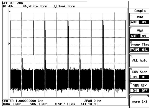
Figure 2-55 Burst Signal in the Zero Span
